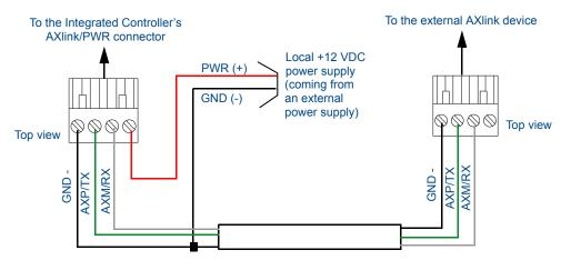
FIG. 6 4-pin mini-Phoenix connector wiring diagram (using external power source)
